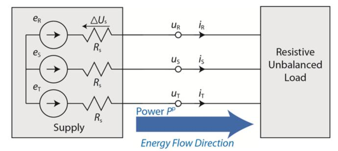
Negative sequence components produce the negative sequence power.
