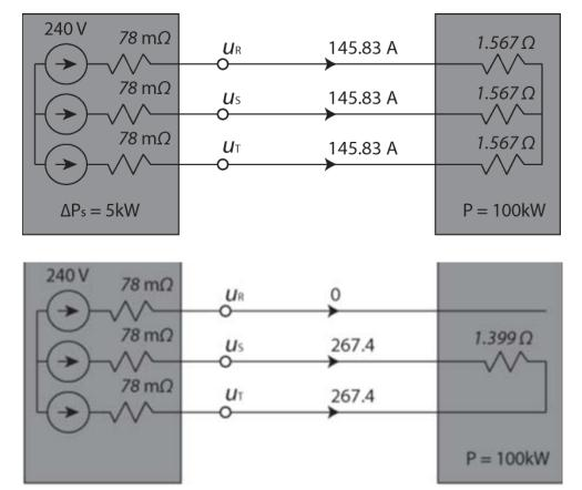
HGLs requires more power than equivalent linear time invariant (LTI) loads from generators.
