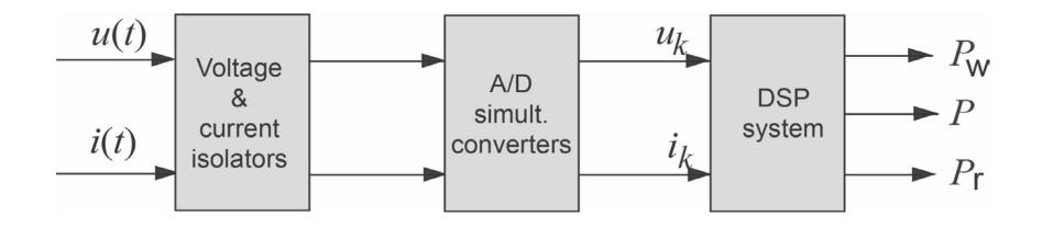
> A/D converters provides simultaneous 14 bit resolution.
